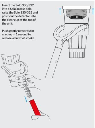
Repeat every 10 seconds without removing the detector for maximum of 1 minute until the detector is activated. On alarm, remove cup to allow particles to disperse.
