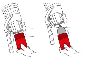
Insert the red cup back into the unit and rotate clockwise until the aerosol starts to release.
