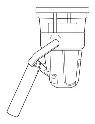
Insert a charged battery baton into the base of the unit and ensure the button locks securely in place.
