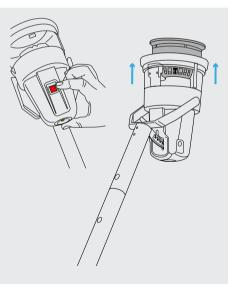
Hold the unit in place until the detector is activated. Solo 460 will revert to standby mode (slow flashing green LED) and the internal blower will cool the heating element for a few seconds.
